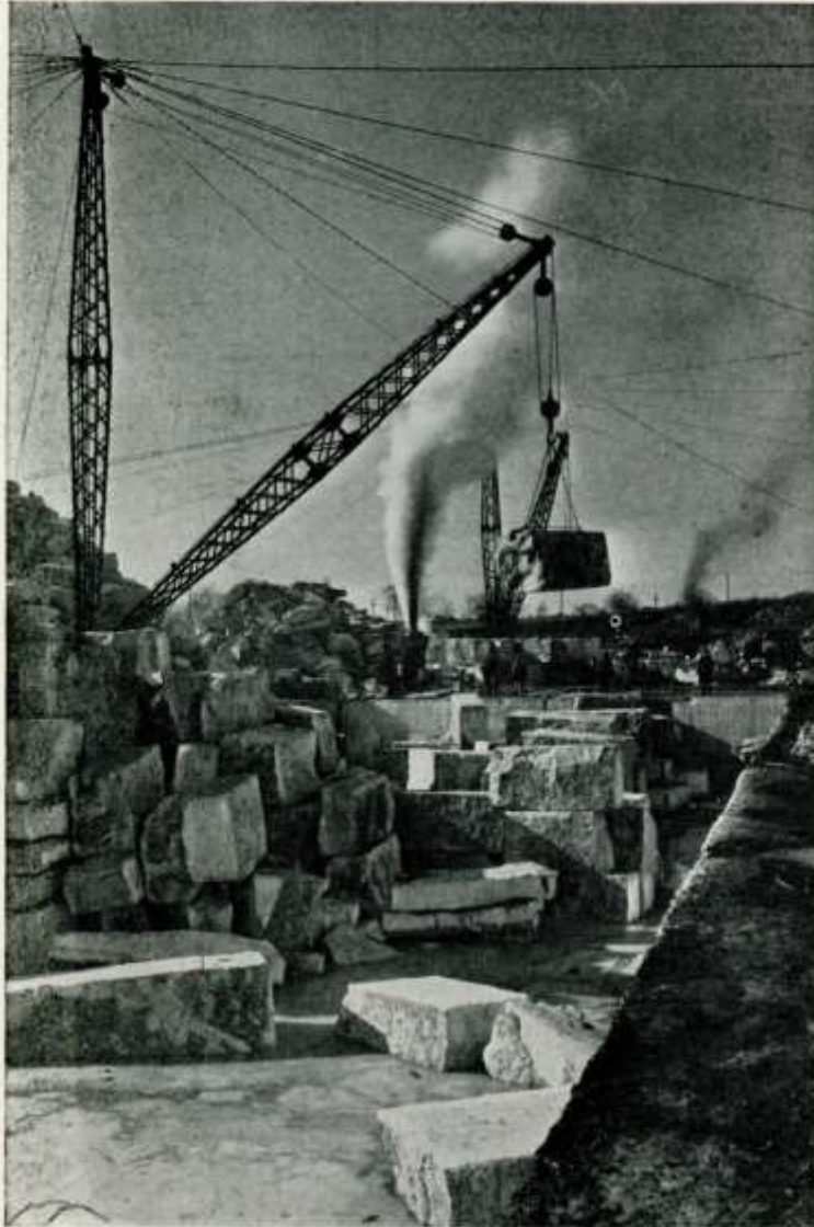
Section of Quarry of F. W. Steadley & Co., Inc., showing derricks and channeling machines and quarry face.
